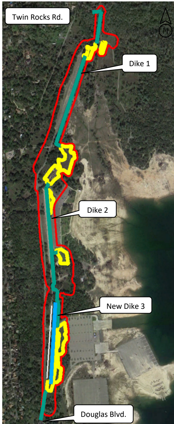
Figure 2-13. Dikes 1, 2, and 3: Limits of construction (red), haul routes (green), staging areas (yellow), existing Dike 3 centerline (white) and new Dike 3 centerline (blue).
